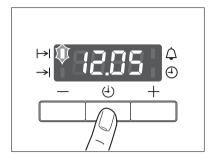
2. Using the + or — button set the desired cooking time.
